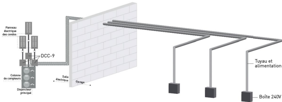
Figure B-7: Example of multiple feeder monitoring devices installed on a meter stack serving a parking garage. Source: MURBLY / RVE.
